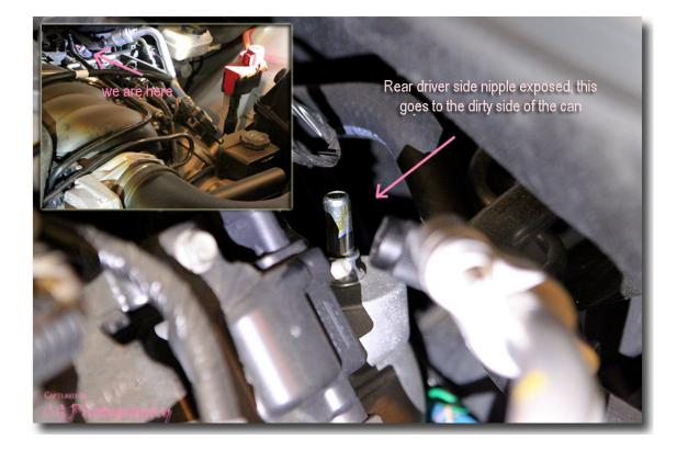
4. Mount the bracket and the can to the bracket.
