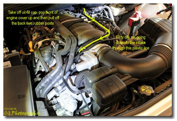
2. Take note of the 3 locations with which you will be working, the ends of the air line, and the mounting bracket bolt.
