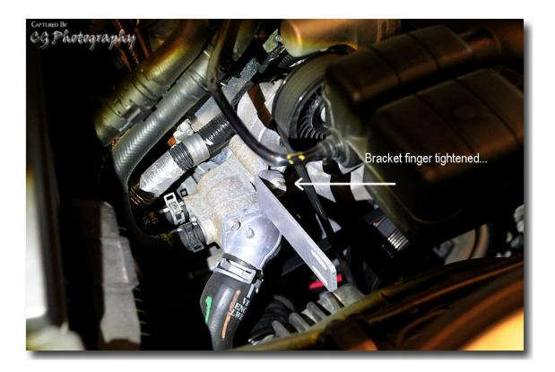
Tighten MN6 bolts and lock collars to catchcan, using lower 2 holes on catchcan, adjust the can on the bolt slots, then tighten down
