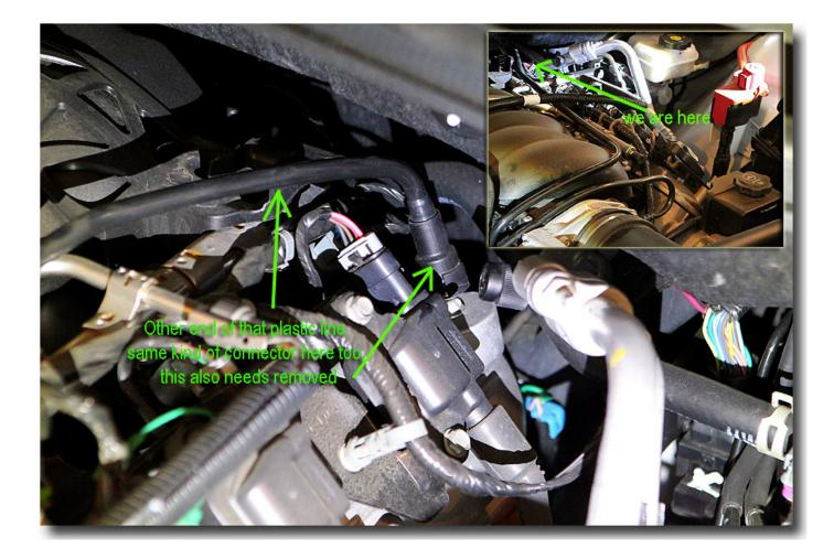
3. Remove the air line connectors from the front and rear nipples. Take note of how these connectors are constructed so that you can remove them with ease. Pictures below show you the end results of what the line looks like and the exposed nipples.
